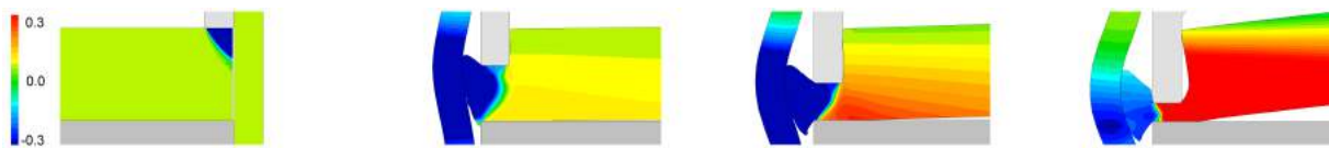
(b) Radial flow velocities for cross-section recess length equal to 1.5 mm and squeezing depths equal to 0, 2, 3 and 4 mm.
