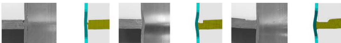
(b) Photographs and finite element predicted geometries of the cross sections of the sheet-tube connections shown in (a).
