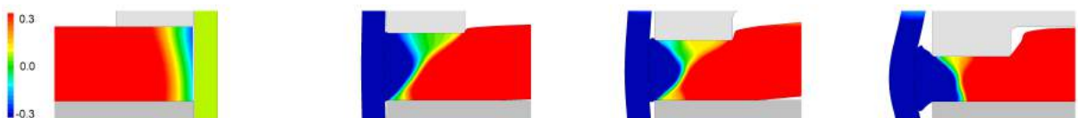
(d) Radial flow velocities for cross-section recess length equal to 5 mm and squeezing depths equal to 0, 0.5, 1 and 2 mm.
