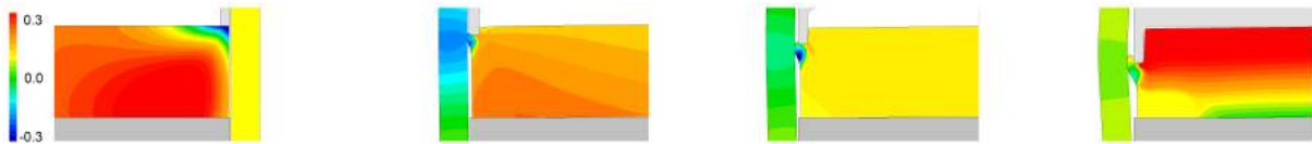
(a) Radial flow velocities for cross-section recess length equal to 0.5 mm and squeezing depths equal to 0, 0.5, 1 and 2 mm.
