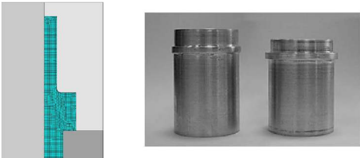
Figure 2.13: Finite Element mesh of Annular Flange and experimental results (Alves et al., 2017).
