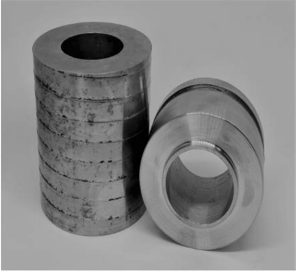
(a) Active components. To the right is the lower die and to the left is the squeezing punch.
